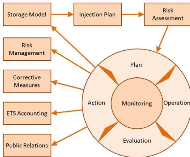
Fig. 5-1: Schematic evolution of site-specific monitoring plans in relation to other elements of CO<sub>2</sub> storage management.
