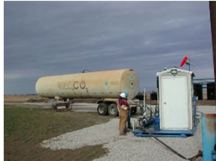
CO2 tank used in a CO2 injection project
