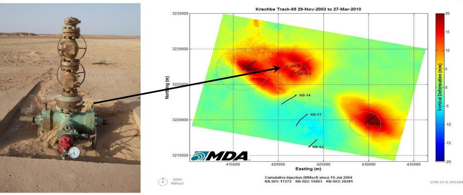
Drilled in 1980 and temporarily suspended (no integrity to gas) 1.5 km NW of KB502  $CO_2$  injector (expected CO2 migration direction) 0.1 tonne  $CO_2$  seeped in 2007 (valve leak – not pressure on gauge) Caused by lack of well & wellhead integrity (physics not chemistry) KB5 now fully decommissioned with  $CO_2$  resistant cement
