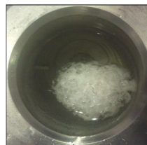
Figure 6. Hydrate formation at the interface of water and free gas
