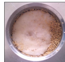
Figure 7. Hydrate formation within the medium grained sediments
