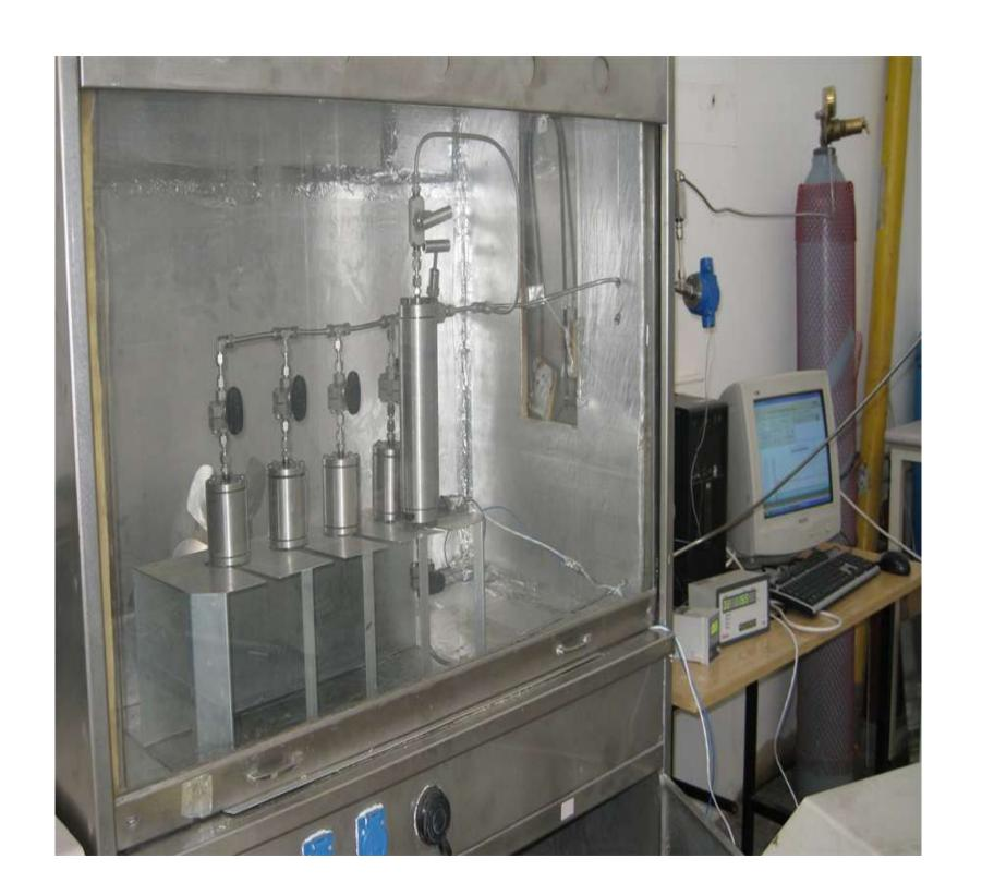
Second step: Portlandite carbonation or cement hydrates  $H_2CO_3 + Ca (OH)_2(s) \rightarrow CaCO_3(s) + 2H_2O$   $H_2CO_3 + C-S-H (Calcium Silicate Hydrate) \rightarrow CaCO_3 + SiO_2$ (gel) +  $H_2O$
