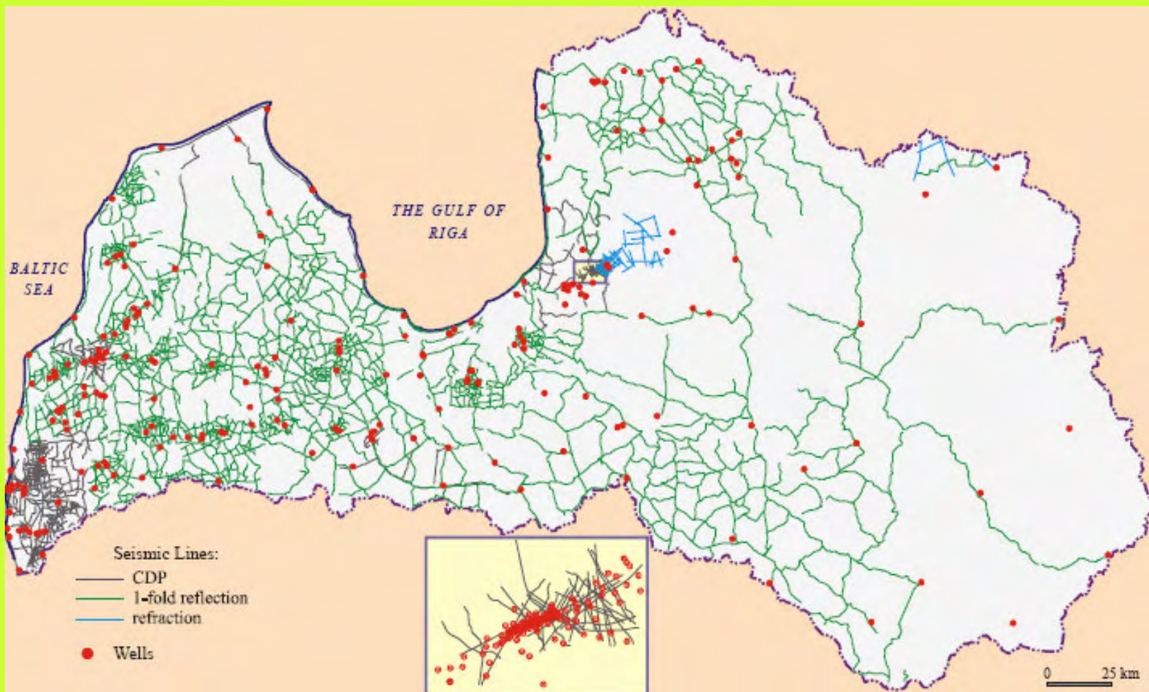
Seismic coverage of the Latvian territory. Green is one-fold reflection, blue – refraction, black – CDP
