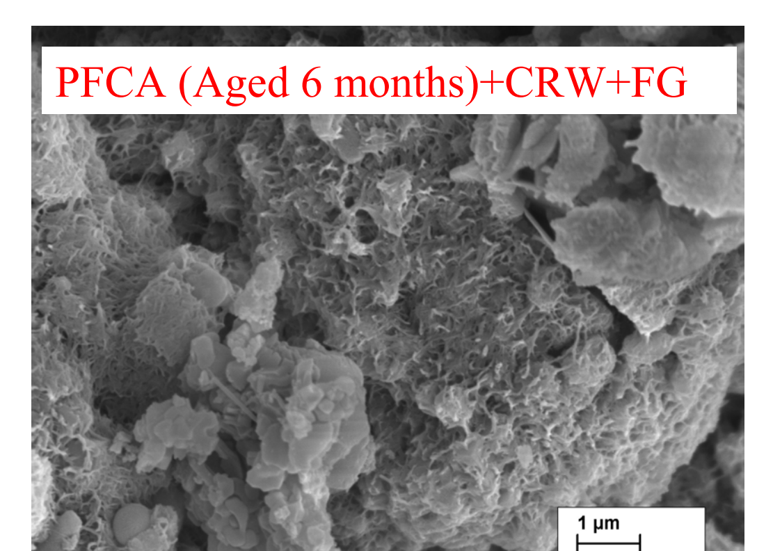
SEM: More porous and permeable product layer (SSA=3,69 m 2 /g)
