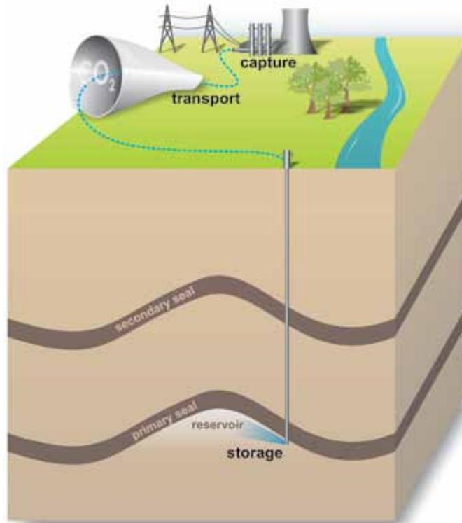
Figure 1: Simplified illustration of a CCS project. CO<sub>2</sub> is captured at an industrial installation, transported via ship or pipeline, and injected into suitable reservoir rock. Multiple sealing formations help to prevent CO<sub>2</sub> from migrating out of the reservoir.
