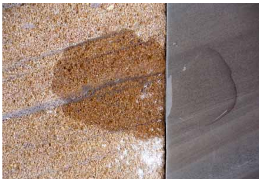
Figure 3: The result of a small test with water as an analogue to the behaviour of CO 2 at large depths. Water infiltrates rapidly into the porous sandstone (reservoir) on the left, but not into the impermeable siltstone on the right (reservoir seal).
