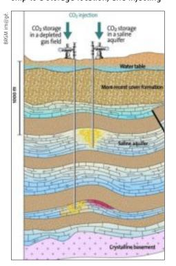
it via a well into a suitable deep geological formation for long-term storage. In doing so, the carbon extracted from the ground in the form of coal, oil or gas is returned back again in the form of CO<sub>2</sub>, making CCS a smart solution that can help avoid the current situation of large CO<sub>2</sub> emissions disturbing the atmosphere and provoking climate change, sea level rise and ocean acidification.
